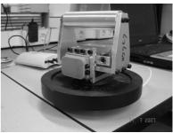
Figure 1. Experimental setup of a handle connected to a mass load, with 3D inertial and force/moment sensors
