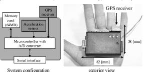
Fig.1 Portable physical activity monitoring unit
