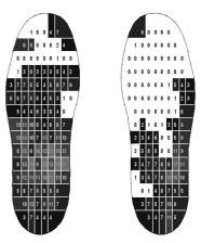
Fig. 1 Pressure sensor layout
